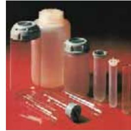
Type HEROLAB polycarbonate tubes transparent Polypropylene tubes translucent. Autoclavable.
